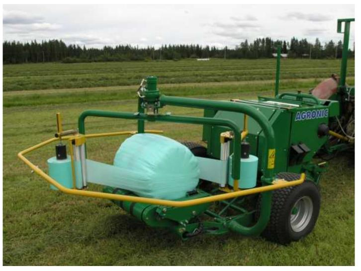
The **AGRONIC W600 COMBI** is equipped with an automatic wrapper that efficiently wraps the material immediately after the material is baled.
