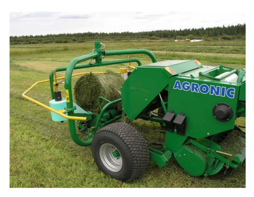
The baler is a fixed chamber baler with a net applicator. The density of the bales is adjustable by a hydraulic chamber lock.
